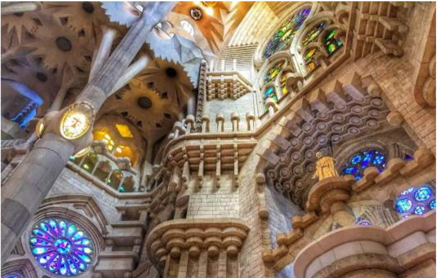
The columns supporting the building were built to mirror trees and branches, each spanning various geometric forms. A simple example is a square base progressing to an octagon, passing to a sixteen-sided form and ending up in a circle. None of the interior surfaces are flat and the level of detail contrasts with the ornate exterior. Every aspect of the building is etched in my memory as a source of inspiration!
